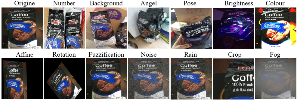
Fig. 4. Data augmentation on an image from our dataset. There is relatively large interference information in the image that the training process can improve the generalization ability and the robustness of the backbone network to deal with jamming information.
